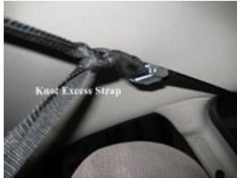
Pull the end of the strap as tight as possible as if you are in a tug-of-war. It is very important that it is extremely tight. When it is as tight as possible, knot the excess strap. The strap will now form two half circle around the roof of your car.
